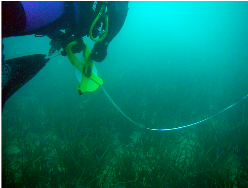
Figure 3. Measuring the degree of burial and meadow patch area in a P. oceanica meadow of the Costa Brava.
