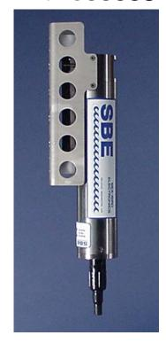
Compensation of the temperature influence on pressure offset and scale is performed by the MicroCAT's CPU.
