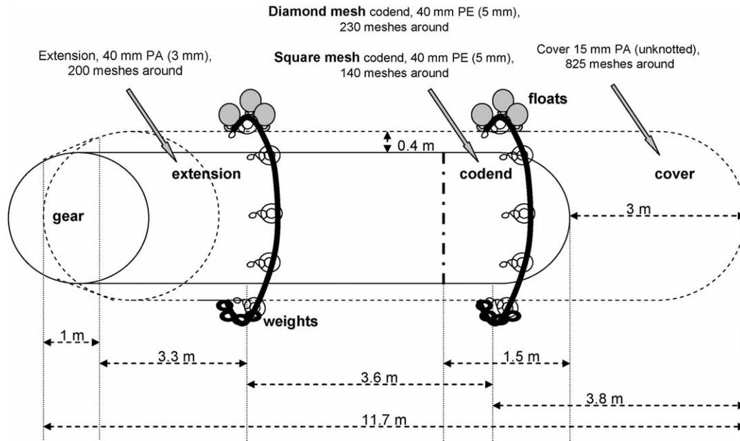
Fig. 2. Schematic illustration of the experimental gear.
